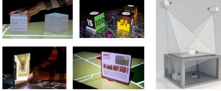
Figure 7: Tangible 3D tabletops. Left side: examples of different uses for 3D and 2D tangible objects on a map. Right side: tabletop system using two top projectors (in order to be able to project on 3D objects) and a bottom projector to display the map on the table. A camera under the table detects the positions of the tangible objects using the markers beneath them.
